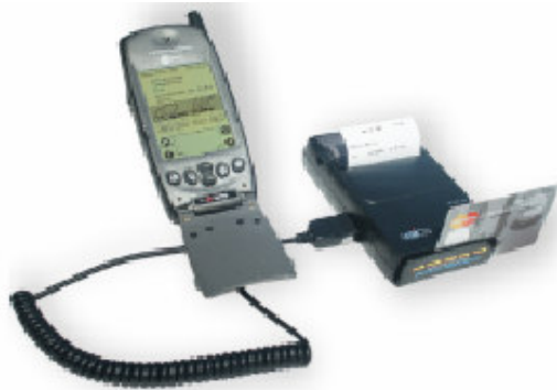
ILLUSTRATION 89 – Connection to a printer-integrated card reader
